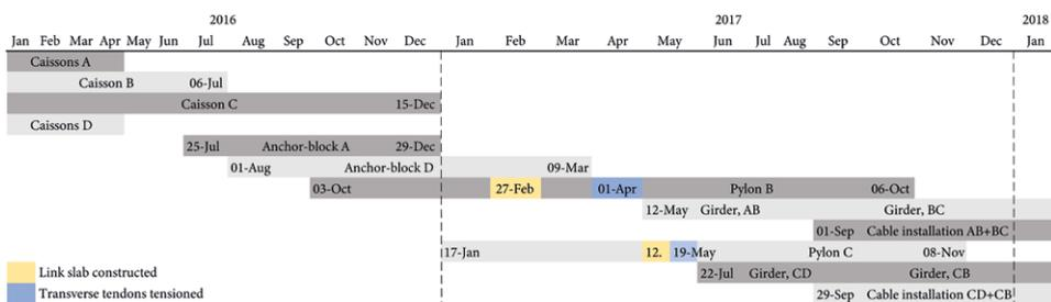
**Fig. 3.1** Overview of the general construction sequence
