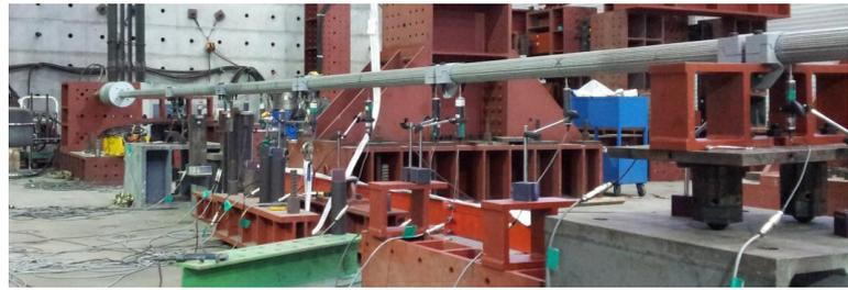
Fig. 1: Deflection measurement test of PWS
