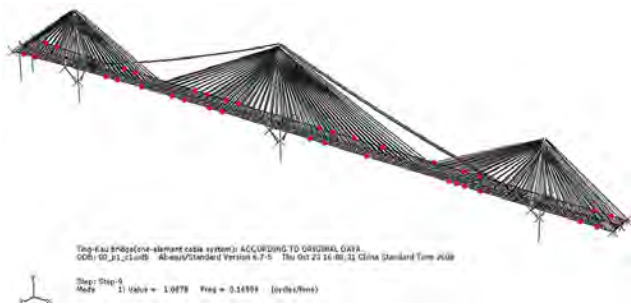
Fig. 1: Final Optimal Sensor Placement for Ting Kau Bridge
