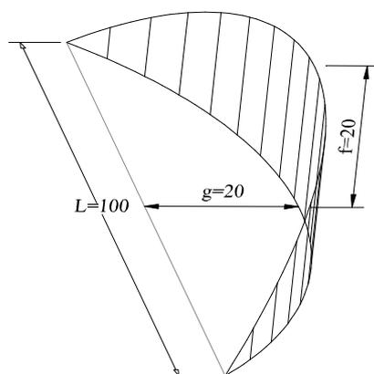
*Fig. 1: Nomenclature and reference values for the models that have been studied for inferior deck arch bridges with imposed curvature*
