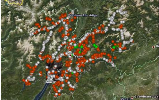
Fig. 1. Distribution of risk associated with an accident due to sub-standard guardrails.
